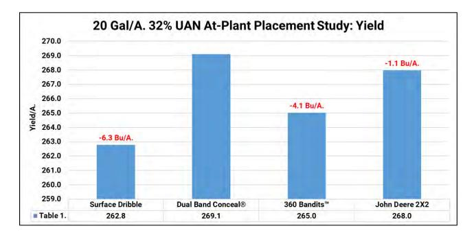
John Deere® 2X2 units proved -1.1 Bu/A. losses compared to the Conceal® system and performed the best relative to 360Bandits<sup>™</sup> and the dribble tubes.
