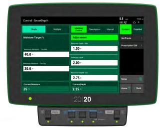
Figure 5. SmartDepth® Customization Screen
