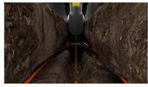
Figure 2. FurrowJet® Tri-Band: Center and Wings
