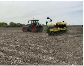
Tire inflations for the John Deere planter consisted of 10.2psi in the front and 11.6psi in the rear of the 942 Fendt® tractor and 50psi in all center and wing tires of the planter. The Momentum® planter was set to automatic weight transfer mode, low tire inflation of 10.2psi in the front tires, 11.6psi on the rear tires of the Fendt® 1050 tractor, and 35psi in the planter tires.
