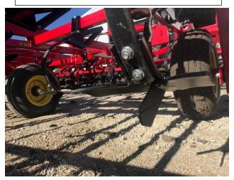
Figure 4. Finish™ Line Sweeps on 9" Spacing
