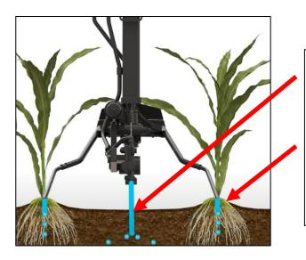
Center of Row Knife and Nozzle High Pressure Knife and Nozzle Injection
