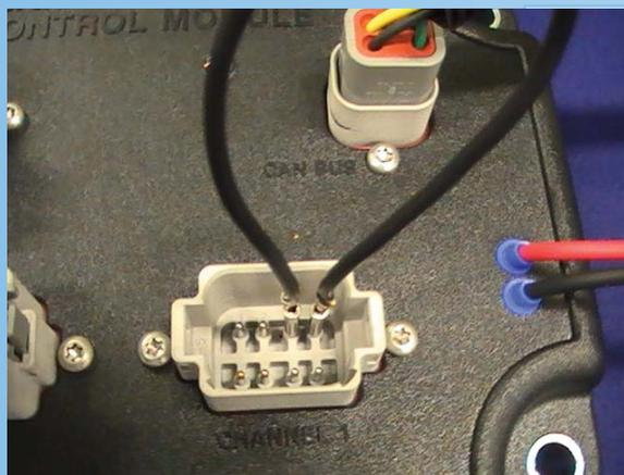
b. If jumping these pins increases the Flow Meter Pulse Count value, then you most likely have an issue with the Control Valve/Flow Meter cable.
